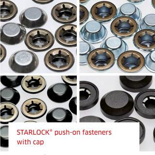
STARLOCK® push on fasteners with a fixed cap are ideally suited to apply at the end of a shaft. The components are thereby secured in place while, at the same time, the cap provides a visually appealing, decorative finish. Both the standard and the deep caps are made of stainless steel; the extra-deep cap is steel with a zinc finish. In addition, caps made of PA 6 plastic in the whole range of RAL colours can be fitted to the push on fasteners. Further individual solutions are also possible.
