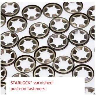
Varnished push on fasteners made of 1.1231 spring steel are part of the standard range. To aid identification, metric STARLOCK\* push on fasteners are varnished brown and imperial STARLOCK\* push on fasteners are varnished blue.
