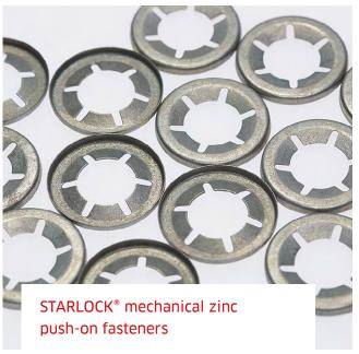
Also made of 1.1231 spring steel, these push-on fasteners have a mechanical zinc finish. They completely rule out the risk of hydrogen embrittlement and offer a very good level of corrosion protection.
